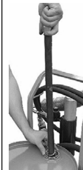
Fig. 3 Raise suction tube fully and rotate until drive dog engages (see fig.1). Keeping tube in raised position rotate clockwise to fully tighten the adaptor into the drum. Lower tube fully into drum.
