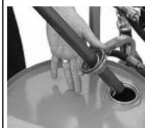
Fig. 2 Insert suction tube and screw adaptor to engage in drum thread. One or two turns is enough.
