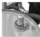
Fig. 3 Raise suction tube fully and rotate until drive dog engages (see fig.1). Keeping tube in raised position rotate clockwise to fully tighten the adaptor into the drum. Lower tube fully into drum.
